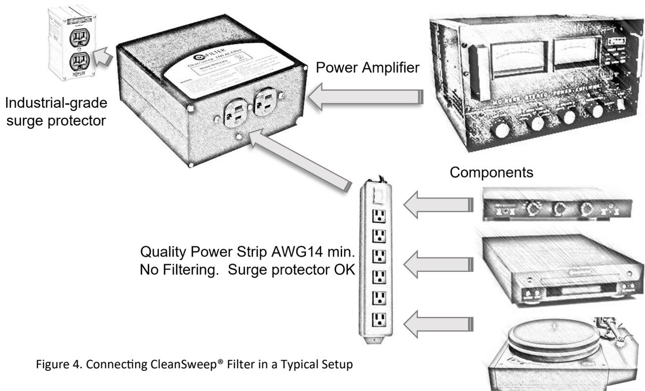
Figure 4. Connecting CleanSweep® Filter in a Typical Setup
