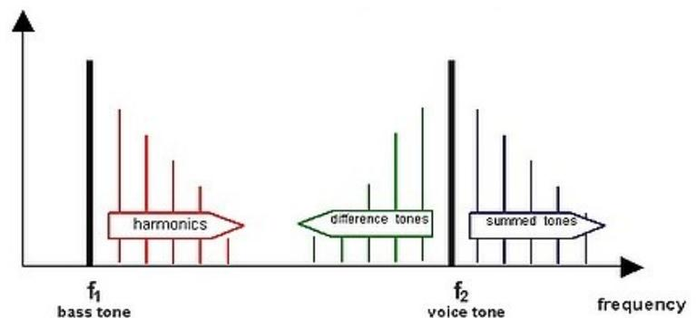
Figure 2. Intermodulation Distortion
