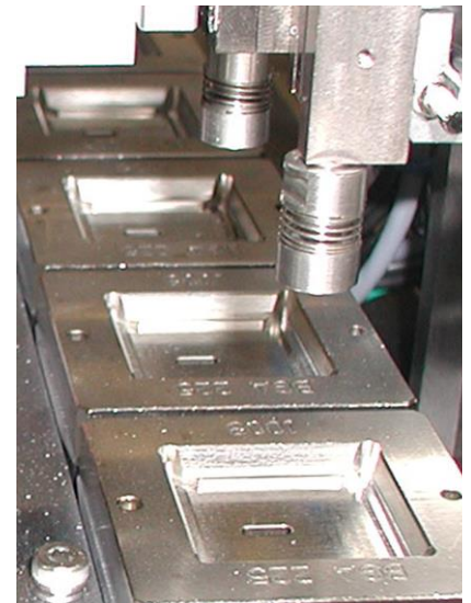
Figure 1: Nozzle and shuttle in an IC handler
