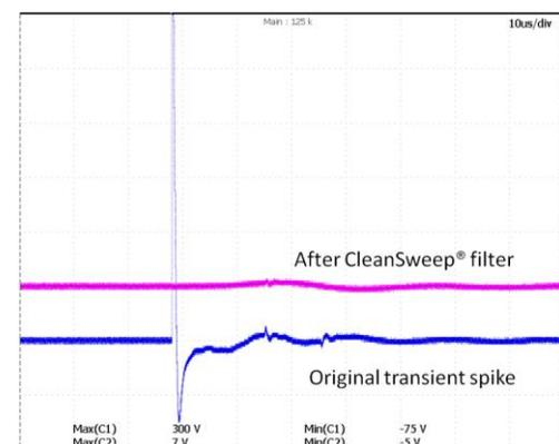
Figure 8. CleanSweep filter suppression performance
