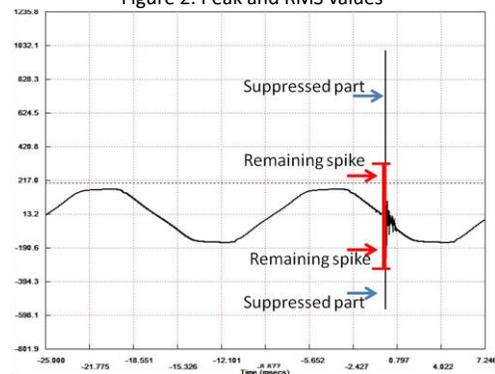
Figure 3. "Suppressed" power line transient
