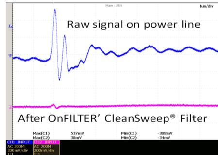
Figure 13. Performance of CleanSweep® filter
