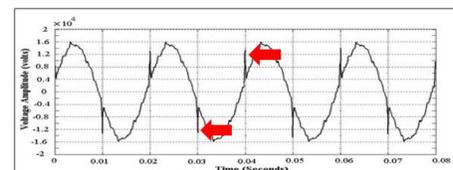
Figure 3. Unsuppressed power line transients
