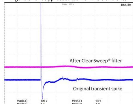
Figure 4. CleanSweep filter suppression performance
