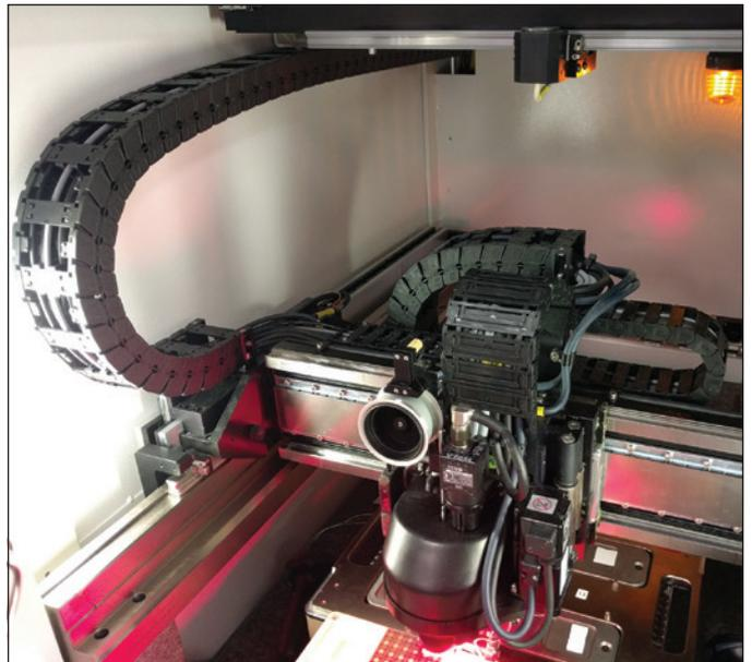
Figure 3: Flex conduit in a typical semiconductor manufacturing tool
