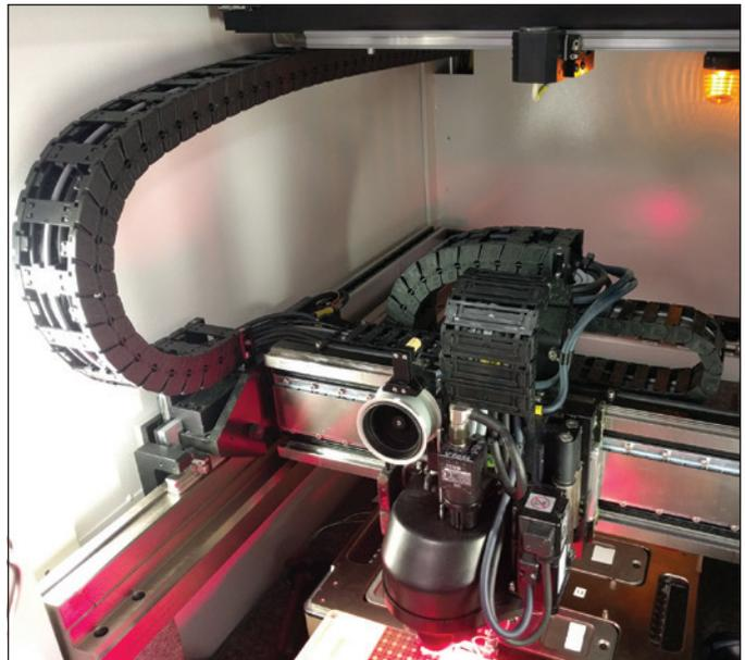
Figure 3: Flex conduit in a typical semiconductor manufacturing tool
